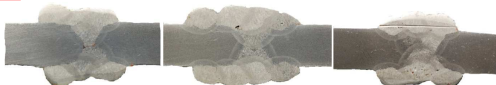
(a) Root opening 3 mm (b) Root opening 5 mm (c) Root opening 7 mm
