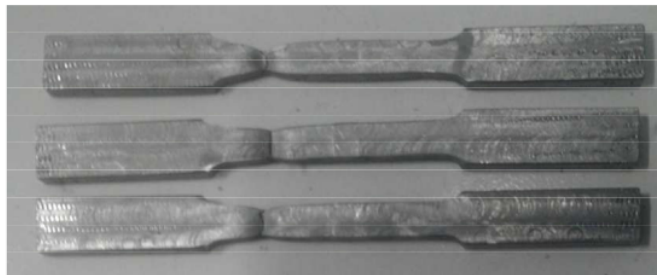
Fig. 7 Fracture location of tensile specimens.
