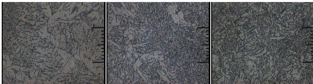
(a) (b) (c) Fig. 4 Microstructure of Welding Zone. (a) Gap 0 mm (b) Gap 3 mm (c) Gap 6 mm
