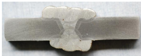
Figure 6. Macrostructure of double side weld metal
