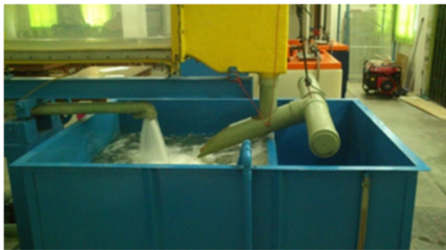
Figure 5 Bend for discharge measurement
